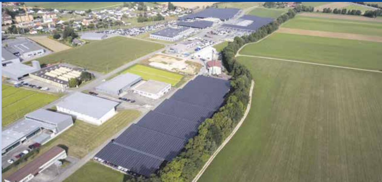
Fig. 5 - Solar power plant Courgenay (JU). GEFCO, EDJ and BKW built Switzerland's presently most powerful solar plant. The installation comprises 23 886 modules built on a site measuring 43 000 m 2 . It corresponds to the size of four and a half football pitches and also houses GEFCO Switzerland's car fleet. The new solar power plant has an installed capacity of 6,7 MWp, which covers an average consumption of over 1 550 households, and is therefore Switzerland's most powerful photovoltaic installation (Photo: ©BKW).
