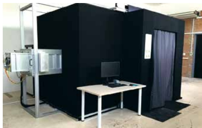
Fig. 3 - CSIR Indoor sun simulator located in Pretoria.
