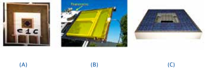
Fig. 4 - CPV cells and modules developed by RSE: (A) CPV MJ solar cell, (B) Test of (Al)InGaP solar cells for luminescence concentrators, (C) new hybrid CPV/PV module.
