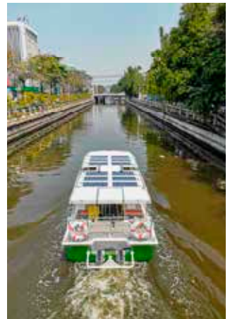
Electric boat service with solar PV installed on its roof in Bangkok (Photo: Arkorn Soikaew)
