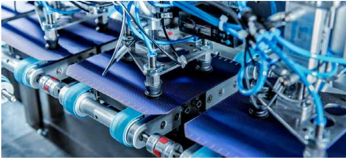
Fig. 6 - Leverage for cost reduction lies in increasing efficiency of modules, the reduction of material costs and high module reliability. An industrial R&D project within the framework of a European cooperation ( SOLAR-ERA.net ) has made significant contributions to these challenges by combining fine-line metallization of solar cells with the cell connection technology from Meyer Burger. On the cell level, silver paste consumption for metallization could be lowered to 5 mg/Watt, which is far ahead in the photovoltaic technology roadmap. With the modules built and tested with this approach, the total module power exceeded by 15 watts compared to commercial 3 busbar modules (Photo: Meyer Burger).
