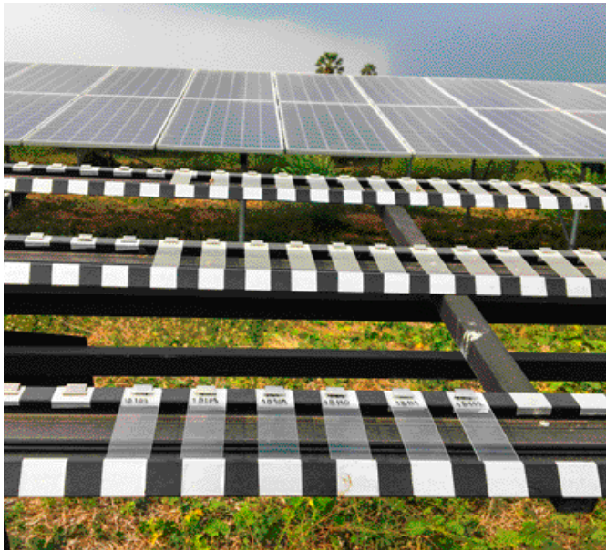
Fig. 2 - A King Mongkut's University of Technology Thonburi (KMUTT) study on the impact of dust on the performance of solar power systems in Thailand (Photo: KMUTT).
