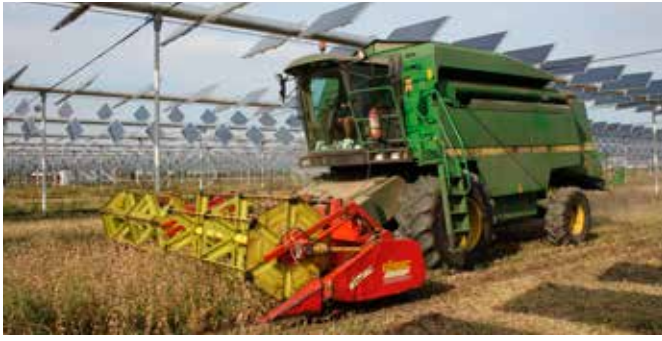
Fig. 2 - REM Tec PV system solution for integration with standard agricultural operation.
