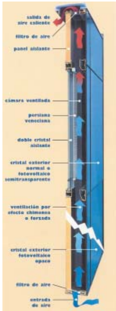
▲ Figure 6.13: Ventilated photovoltaic curtain wall. Source: TFM, Spain.
