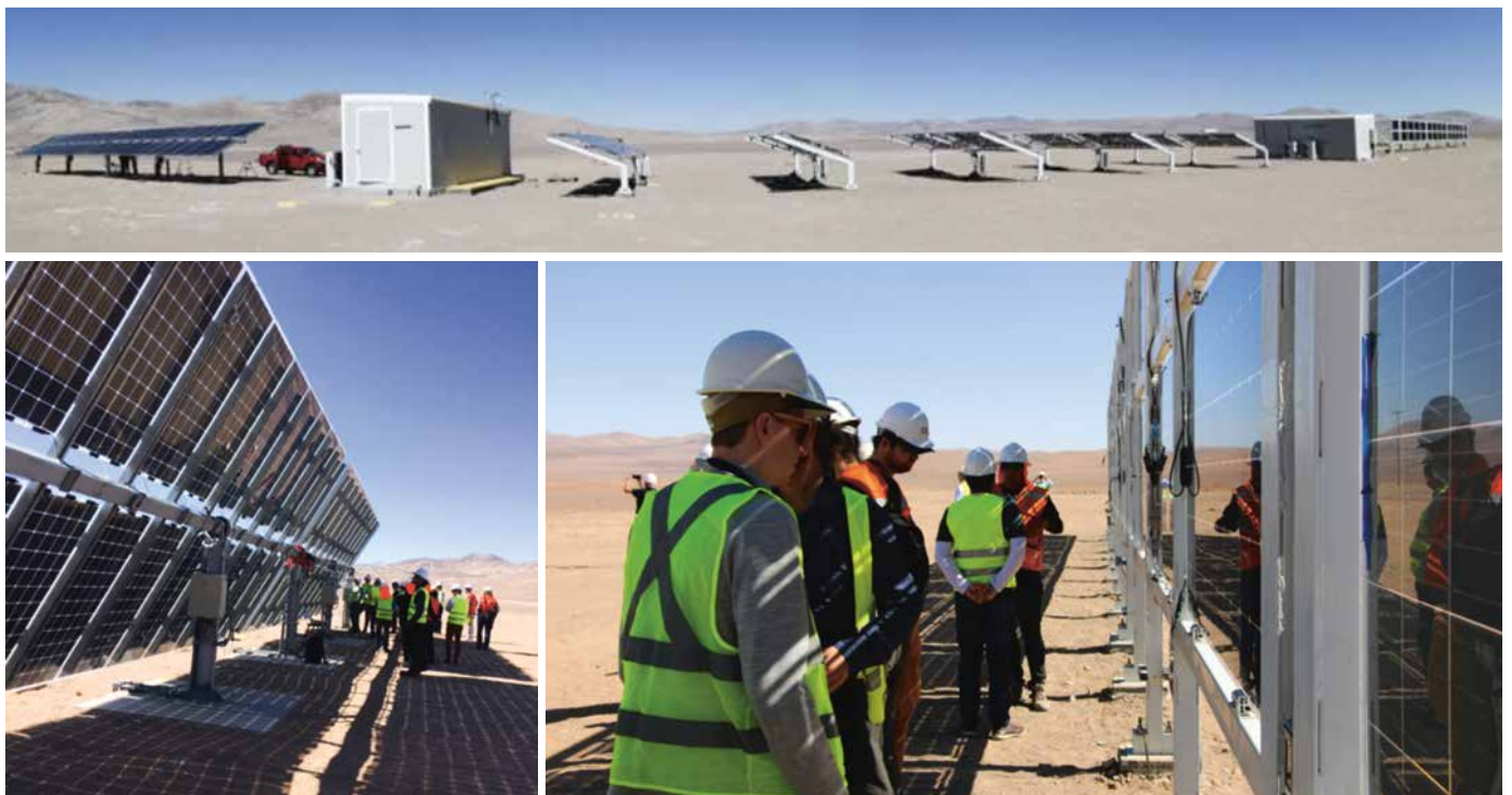
Fig. 4 – First version of Atacama module (ATAMO) installed at the Antofagasta Solar Testing Platform developed by ATAMOSTEC Consortium and CEA-INES and ISC Konstanz technology partners.
