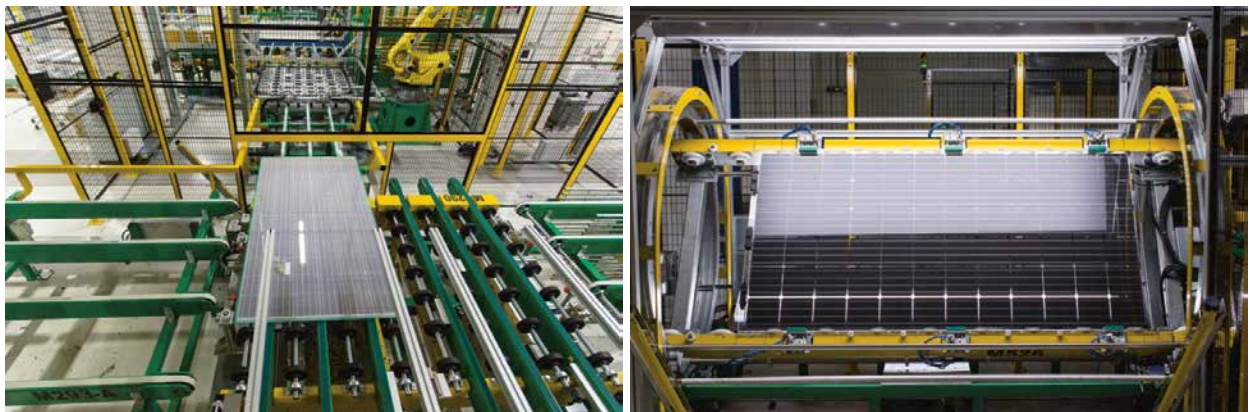
Fig. 5 – EGP 3SUN PV module factory: HJT bifacial module assembly line.
