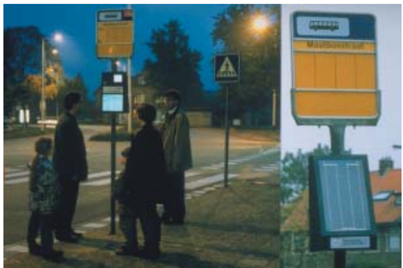
▲ Figure 1.5 a+b: Display at the station powered with photovoltaics - day and night. Source: a) Fraunhofer ISE Freiburg, Germany and b) Ecofys, The Netherlands.
