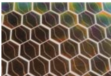
▲ Figure 6.8 a-c: Different solar cells were designed within the European project BIMODE. Colours and forms (here: hexagonal) can vary according to the architectural and aesthetic requests. Source: Astrid Schneider, Germany.
