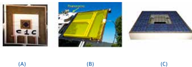
Fig. 4 - CPV cells and modules developed by RSE: (A) CPV MJ solar cell, (B) Test of (Al)InGaP solar cells for luminescence concentrators, (C) new hybrid CPV/PV module.
